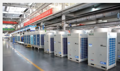
Air conditioning Outdoor unit production line
