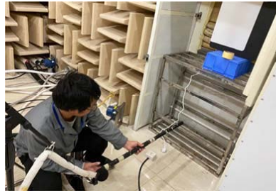
1.5M meters in front of ventilator
