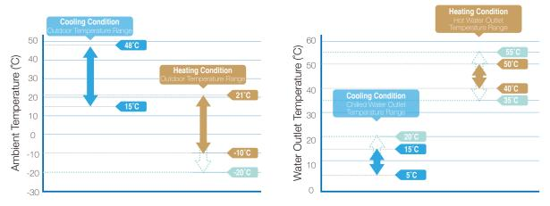
Note: The solid colour marks are the operating range of normal temperature type equipment. The dotted line marks are the extended operating range of low-temperature type equipment.
