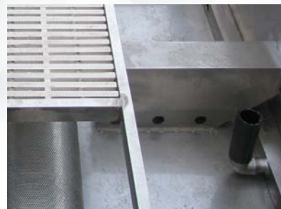
All stainless steel material, water level control and overflow filtration system
