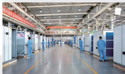
Assembly area of combined air handling unit
