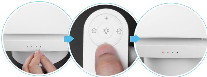
When the other ventilator is powered on and switched off, use the needle to poke the reset button and press it twice quickly. The green LED will flash slowly, the unit enters the matching mode.
