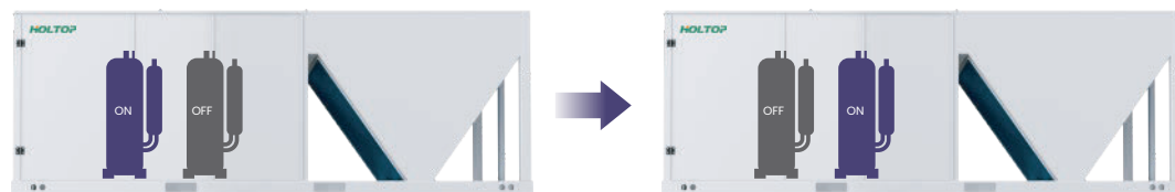
Compressor Alternative Operation
