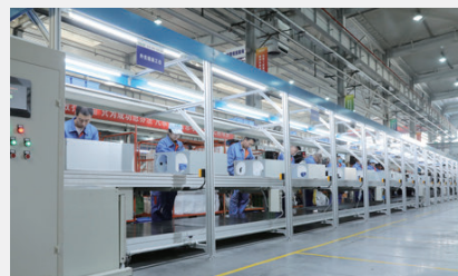
Assembly line for standard ventilation unit
